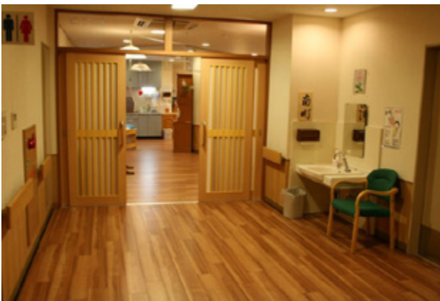
Cushioning floor: This type of floor offers fracture risk reduction for residents and fatigue prevention for the staff.
