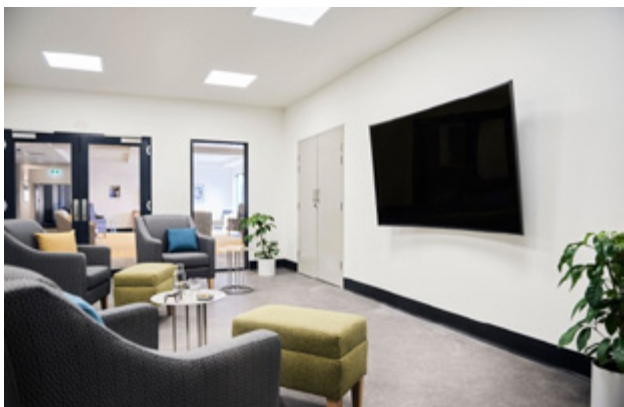
The TV room is separated from the lounge room to avoid loud noises. Black skirting was selected to give contrast between wall and floor. Residents use doors that have black frames while white frames signify no use.
