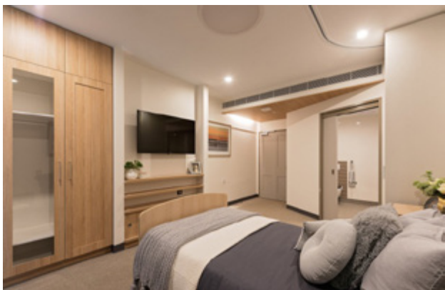
The resident bedroom has a clear line of sight from the bed to the toilet and a clear panel in the wardrobe to assist older adults living with dementia.
