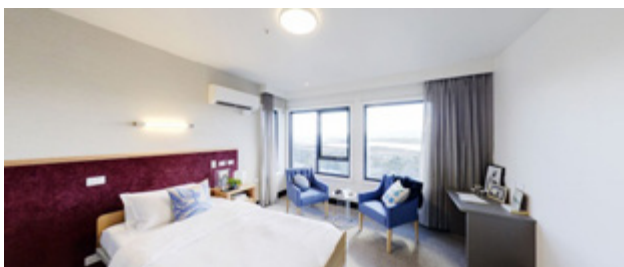
A resident's bedroom. The blue chairs and small white table are examples of furniture the residents can bring. There is space to allow general furniture to be installed. Again, black skirting to identify wall edge and black window frames to windows to define the views. Plain carpet so items can be found.
